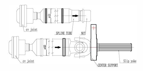
2. WHEN FITTING THE PROPELLER SHAFT TOGETHER, MAKE SURE THAT THE MARKS LINE UP WITH EACH OTHER. THE ARROW OF THE FRONT PROPELLER SHAFT MUST BE ALIGNED BETWEEN THE ARROW ON THE REAR PROPELLER SHAFT.
