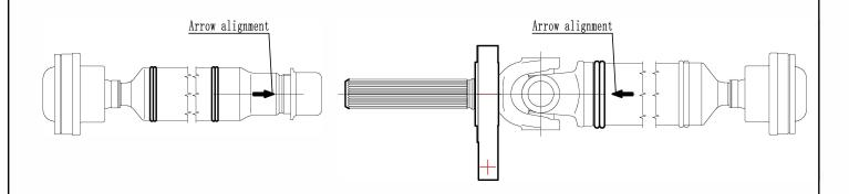
3. SCREW THE NUT TO THE END BY HAND WITHOUT TIGHTENING, MOVE THE SPLINE TUBE TO THE POSITION (USE SPANNER TO LOCK THE NUT.
